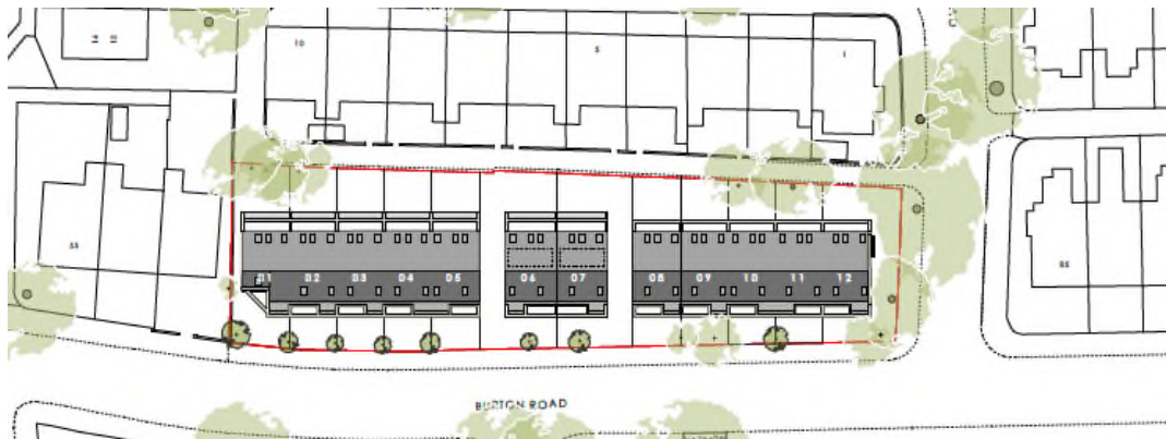
Site layout drawing showing building line relationships between the proposed site and existing properties
